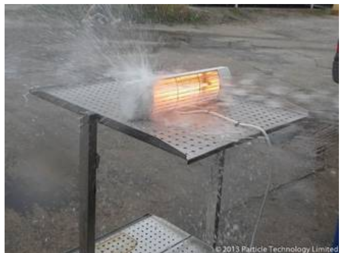
Figure 2 - HLW 15 during IPX6 Water Test
